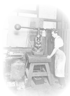
Die sinking the individual lead matrices used in the form
