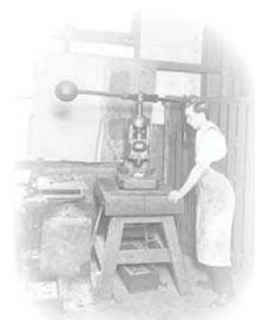
Die sinking the individual lead matrices used in the form
